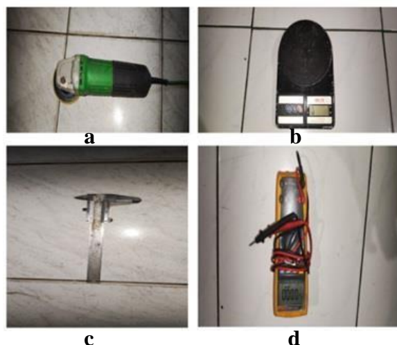
Gambar 15. Equipment, a. Gerinda tangan, b. Timbangan digital, c. Kaliper, d. Multimeter
