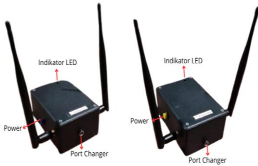
Gambar 3. Hasil implementasi Repeater LoRa LoRa Ebyte E220-400T22D
