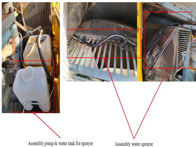
Figure 8. Installation of water sprayer on bulldozer.
