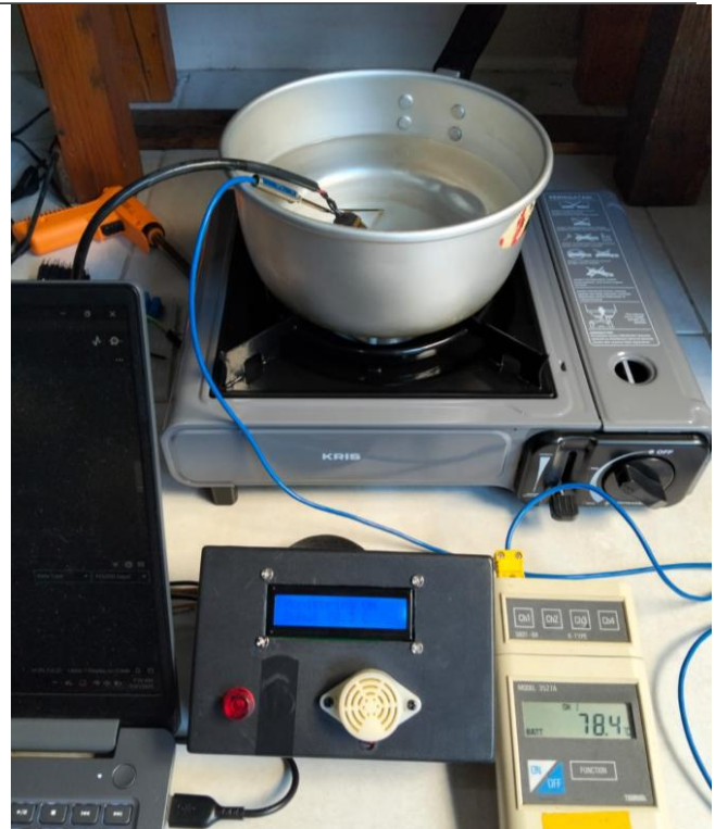
Figure 9. Temperature Sensor Test.
