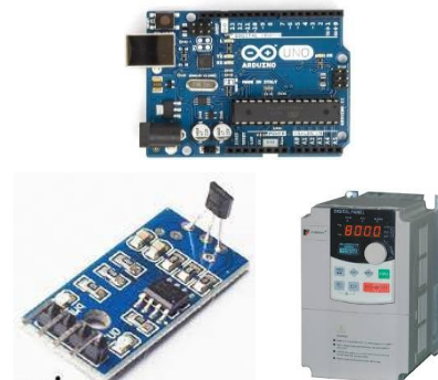
Gambar 1. Mikrokontroler, Sensor hall effect dan Variable Speed Drive (VSD)
