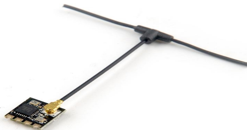
Gambar 9. Antena Telemetri dan Receiver Happymodel ExpressLRS ELRS Nano 2.4GHz EP1/EP2
